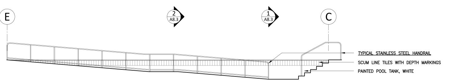
5 LAP POOL ELEVATION - RAMP AND STAIR
